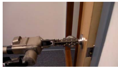
10. Gripper Pulls Door Open by Backing Up Base
