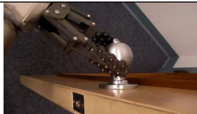
14. Gripper is at limit of grip; different conditions would have seen gripper release by now
