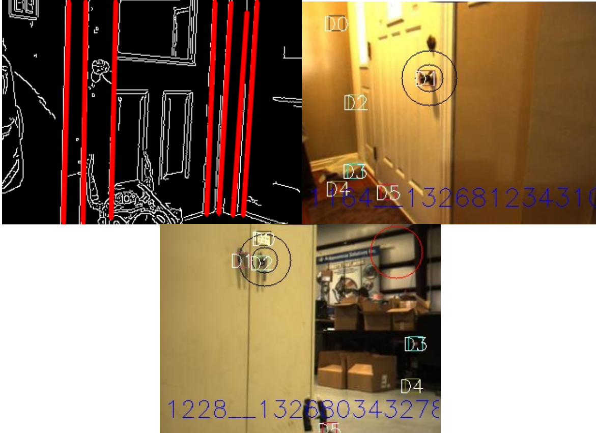
Figure 6: Top left image shows edge detection highlighting candidate wall corners and door edges. Top right and bottom show examples of correctly classified door knob regions
