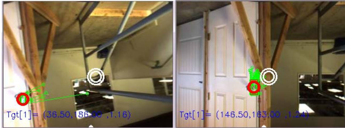
Figure 7: Door Tracking: Red circle indicates knob center, and white is target location to servo towards
