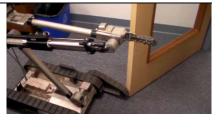
18. Robot driven up until "flipper" can move door aside
