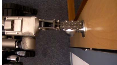
5. Gripper Slips off; Lower Finger is Hitting Flange
