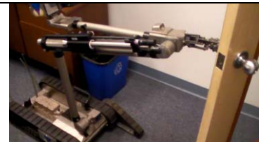
12. As knob angle increases, base adjustment necessary (no compliance at attachment to arm or at grips)
