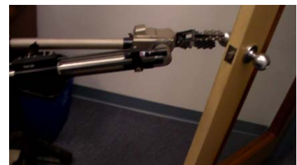
15. Gripper opens and door (unlatched) left slightly ajar
